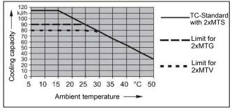
Note: The limit curves for the heat exchangers exchanger PTG, PTV or MTV apply to a dew point of 40 °C.
